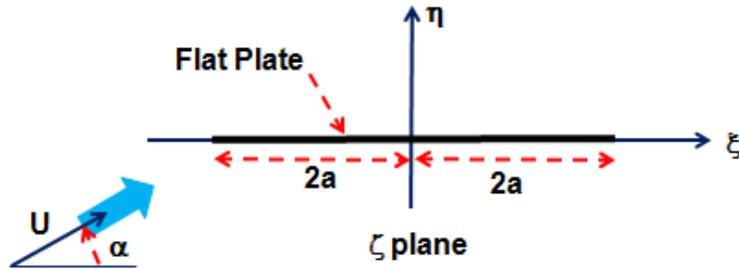
Figure 2:  $\zeta$ -plane for the flow around a flat plate at an angle of attack.
