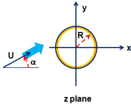
Figure 1:  $z$ -plane for the flow around a flat plate at an angle of attack.
