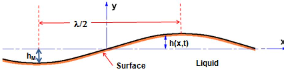
Figure 1: Notation used for gravity waves on an otherwise horizontal liquid surface.
