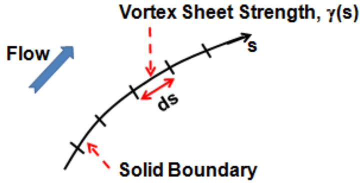
Figure 2: Section of the solid boundary of a planar potential flow.
