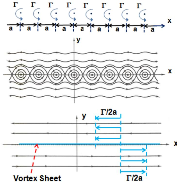
Figure 1: Infinite linear distribution of free vortices of circulation,  $\Gamma$ , and spacing,  $a$ , (top), the resulting streamlines (middle) and the vortex sheet flow as seen from afar (bottom).
